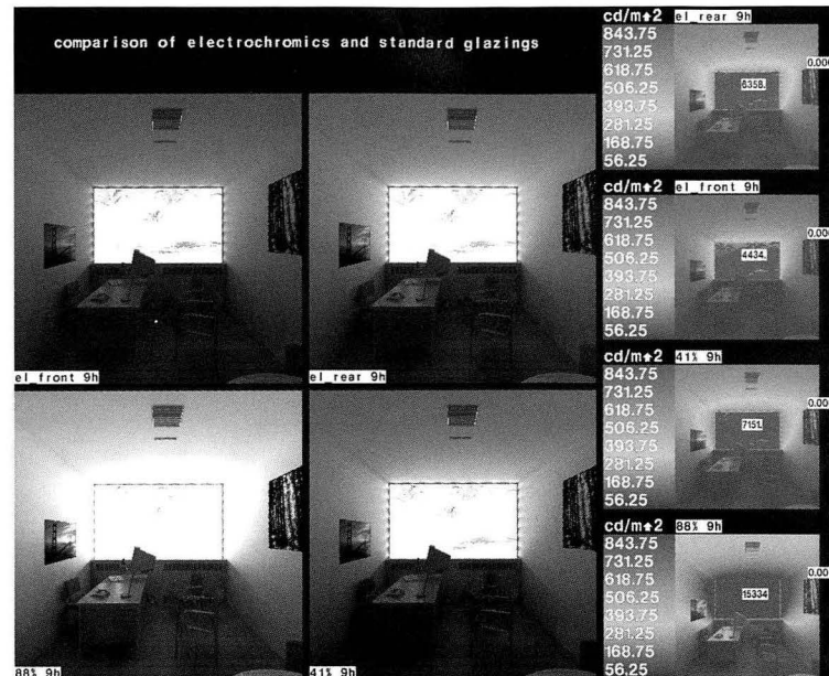
Simulation tools, such as these RADIANCE ray tracing images, compare visibility of a computer screen with conventional clear glass (lower left), tinted glass (lower right), and electrochromic glass (top left), using two different control strategies.
