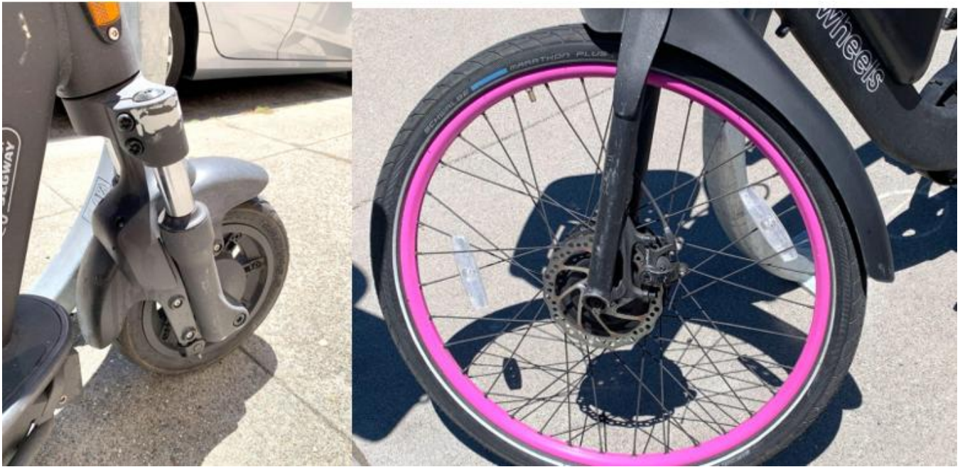
Figure 14. A) E-scooter drum brake vs. B) E-bike cable-actuated disk brake
