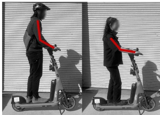
Figure 11. Example of 6' tall rider and 5' tall rider highlighting handlebar height, elbow position, and hand position on a SPIN e-scooter
