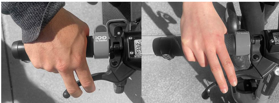
Figure 12. Photo demonstrating how large & small hands can reach a brake lever in its most relaxed position.
