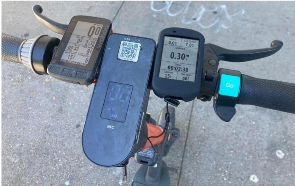
Figure 9. Documentation of GPS computers mounted on a Spin e-scooter during testing
