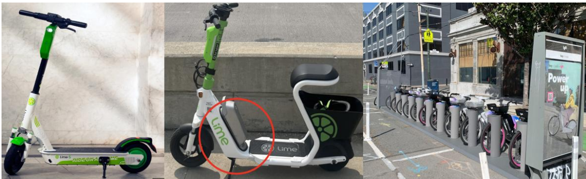
Figure 15. Battery in frame (left), swap out battery (middle), kiosk charging station (right)
