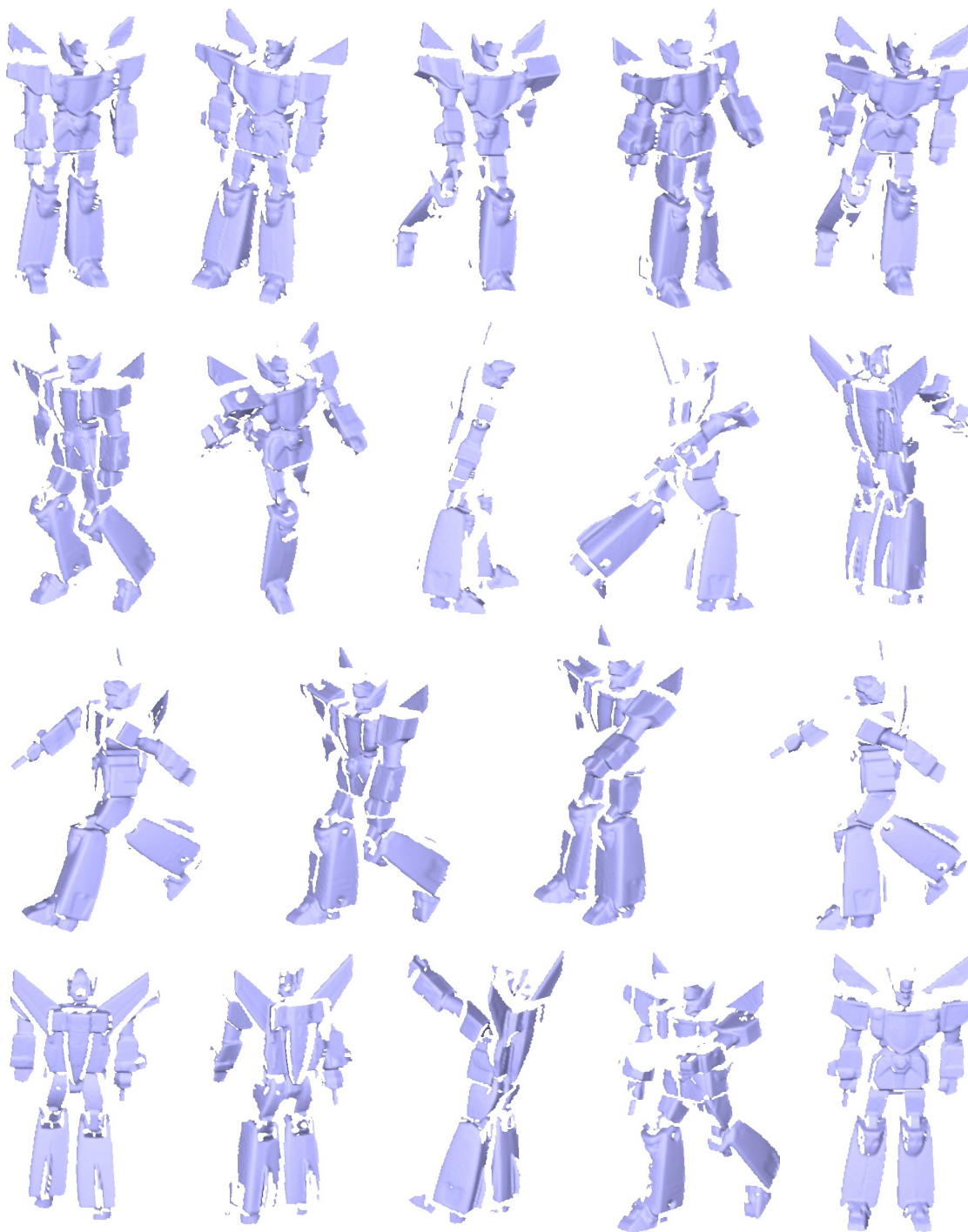
Figure 6.1: Selected range scans from the 90 frame robot sequence. Our goal is to automatically align all of these scans to a common location and a common pose. Data from Pekelný and Gotsman [2008].
