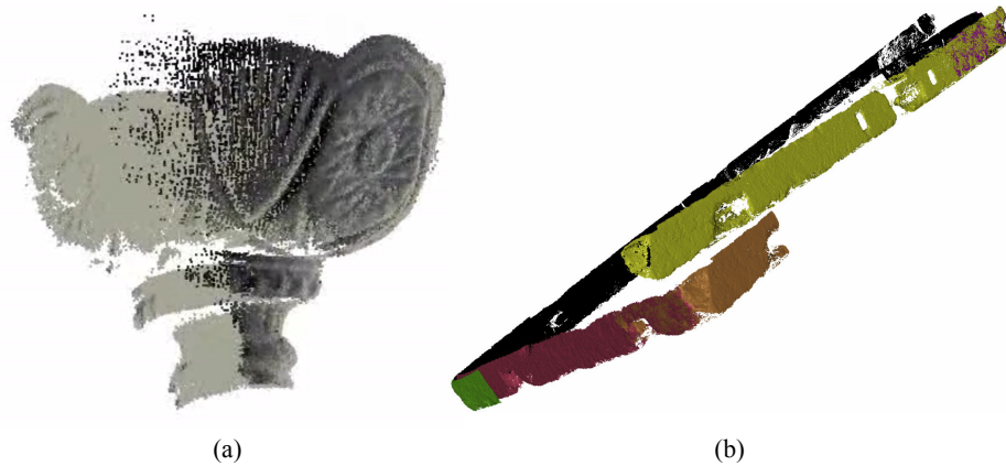
Figure 3.3: Examples of accumulation error using a sequential alignment strategy. In both examples, the range scans wrap around the object and should form a closed ring. (a) We see that the alignment error accumulates and the vase “twists” upwards. (b) Here the first and the last scans do not align well as a result of accumulated error. From Rusinkiewicz et al. [2002]; Brown and Rusinkiewicz [2007].
