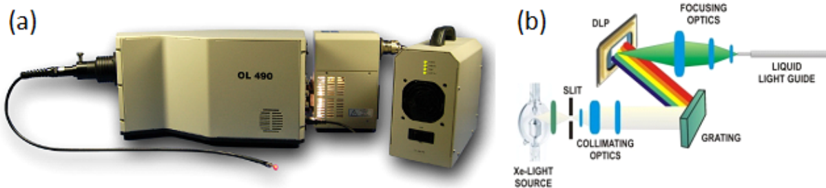
Figure 5.4: A visual of (a) Gooch and Housego’s OL-490 Agile Light Source and (b) a diagram of the mechanics inside the machine.
