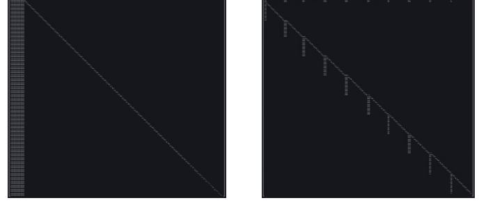
Fig. 1. The sparsity pattern of the equality constraints of typical PTDF model (4) in the left and decomposed PTDF model (9) in the right for case20758_epigrids . The left figure shows the non-zeros of equalities (4c) and (4d) with 33,344 rows, 35,517 columns, and 65,933,978 non-zeros. The right figure shows the non-zeros of equalities (9c), (9d) and (8b) after substituting for the power injection using (9b) with 34,005 rows, 36,168 columns, and 8,743,139 non-zeros.
