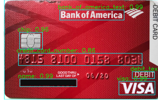
FIGURE 3.8. Output of the object detector of the BIN consistency and expectation check. The model correctly identifies issuing bank, the card network (Visa), card type, chip, name, and card number. These extracted features are correlated with the data of the card BIN to identify any inconsistencies.
