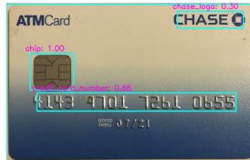
FIGURE 3.14. A BIN inconsistent fake card image caught by the BIN consistency and expectation check. The card shown in the image starts with a 4 and should thus have the Visa logo. The BIN (first 6 digits) of the card is also not from Chase, and thus, a Chase logo should not be present. The BIN check detects both inconsistencies, showing that it would flag such a card as fake.
