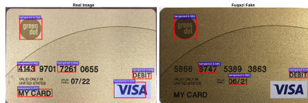
FIGURE 3.7. Tampering regions determined by the Faster R-CNN based model [136] on a real image (left), and Fugazi fake (right). Not only does the model fail to detect the tampered regions in the Fugazi fake, it also mistakenly detects untampered regions on both images.
