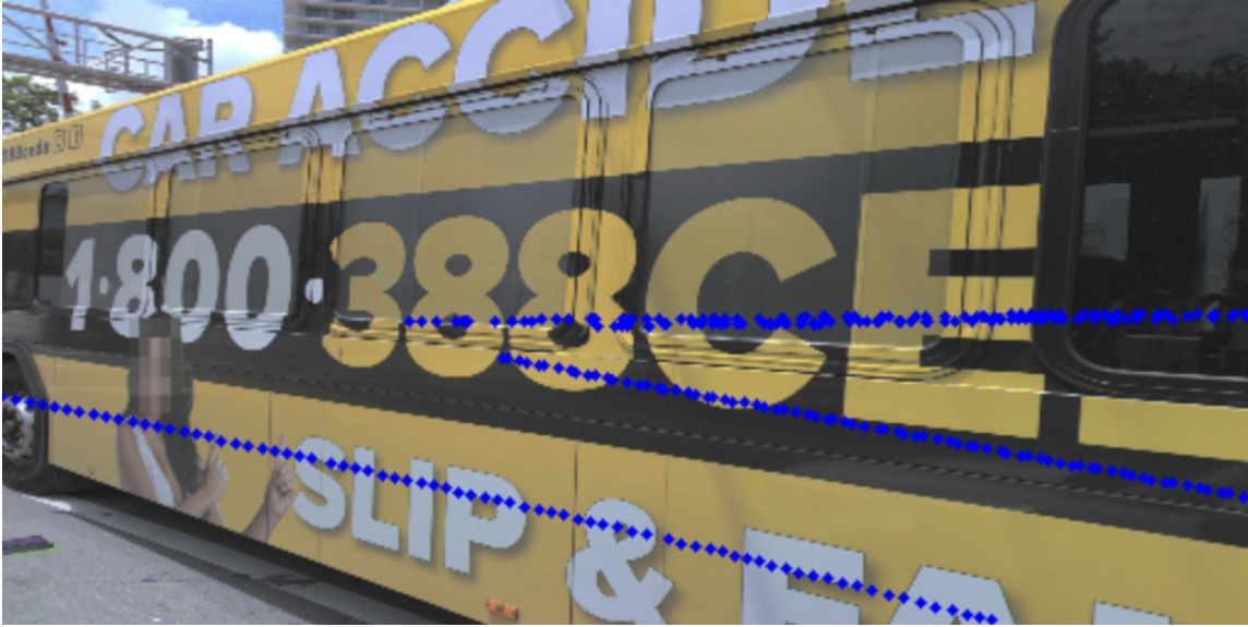
Figure 4.5: Data sample generated by the automatic labeling process without explicitly modeling occlusion. In this scenario, a bus is fully occluding centerline features.
