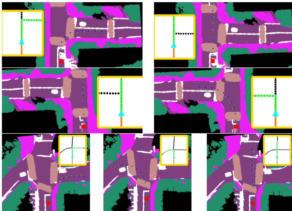
Figure 3.8: Various visualizations from the IntersectionScenes dataset using the SPF graph encoder. Each row represents an intersection with different global plans (yellow boxes). Groundtruth labels are denoted by blue waypoints and predictions by green waypoints.
