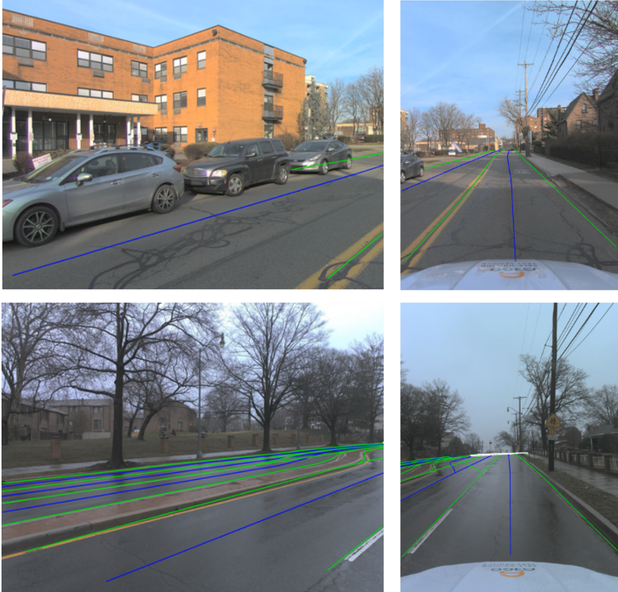
Figure 4.1: In contrast to traditional lane detection tasks (shown in green), our work explores an approach for centerline feature prediction, as denoted by blue lines. The approach leverages automatic label generation to process a large image dataset from an urban driving scenario with 2D and 3D ground truth information.
