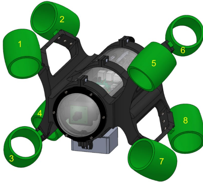
Figure 5.1: CAD model of entire ROV with numbered thrusters
