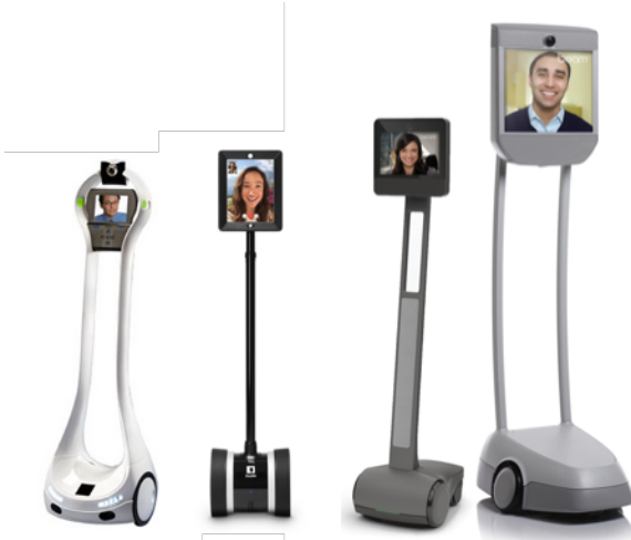
Figure 3. Four commercially available telepresence robots (height in inches): VGo (48”), Double (47-59”), Beam (53”), and BeamPro (63”).
