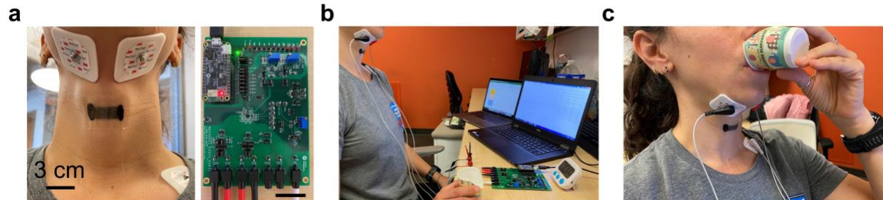
Figure 2.4. On-body experimental set-up. (a) A close-up image of the strain and sEMG sensors on the throat of the participant and the MAX30001 Evaluation kit used in the experiments. Scale bar is 3 cm. (b) The photograph shows the testing set-up where the sensors are connected to the Evaluation kit which is connected to a laptop, and the participant is seated in a relaxed position before instructed to swallow water from the cup. (c) The image captures the participant being instructed to swallow the known volume of water.
