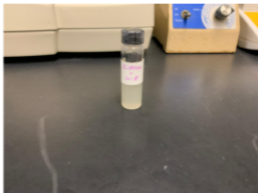
Figure #1 ZnO and Liposome solution in methanol and isopropanol
