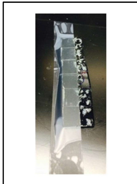
Figure 1.7. Digital photograph image of aqueous 2M HCl and zinc powder reacting to etch away the exposed fluorine-doped tin oxide.
