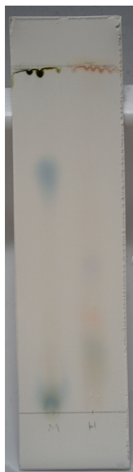
Figure 3-4. Hot water extraction vs methanol extraction of isatan B. Left: I. tinctoria leaves were extracted using 5 parts methanol with 0.1% formic acid. The blue spot at R_f \sim 0.70 is consistent with isatan B. Right: I. tinctoria leaves were extracted using 5 parts water with 0.1% formic acid.
