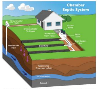
ease note: The ends of the chamber system lines are open for illustrative purposes only. In reality, and when properly installed, these lines are closed at the end. Septic systems vary. Diagram is not to scale.
