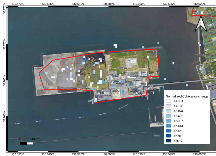
Figure 4.19: Normalized coherence change at the artificial island to the west of Kumamoto City
