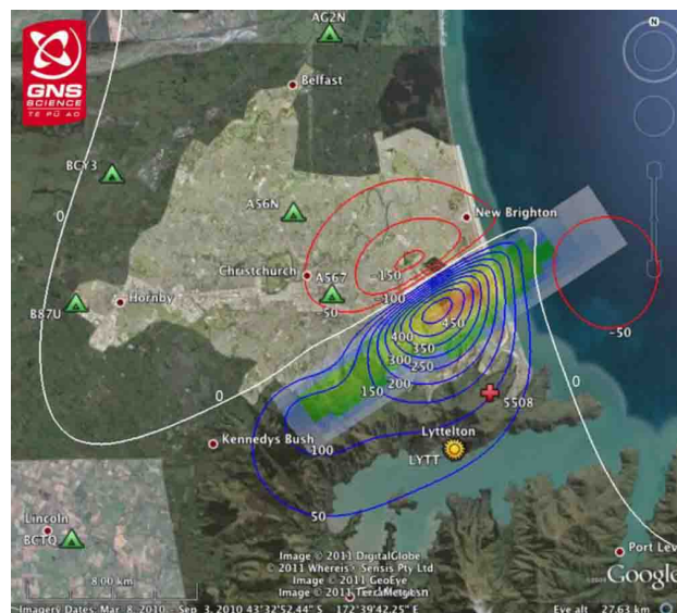
Figure 3.16: Preliminary model of the southeast-dipping fault (rectangular area) that ruptured across the southern part of Christchurch and northern Port Hills during the 2011 Christchurch earthquake. The red, green and yellow symbols show some of the GPS stations whose displacements were used to derive this fault slip model (GNS Media Release, April 2011).
