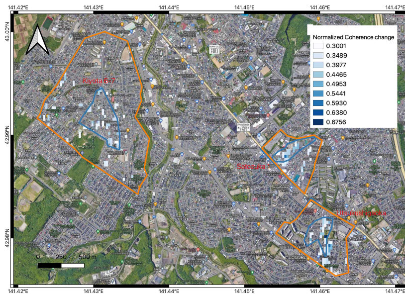
Figure 5.12: Normalized coherence change map in Sapporo City where flow-failure occurred (Liquefaction-damaged areas bounded in blue lines are from Ishikawa et al. 2021 [36])
