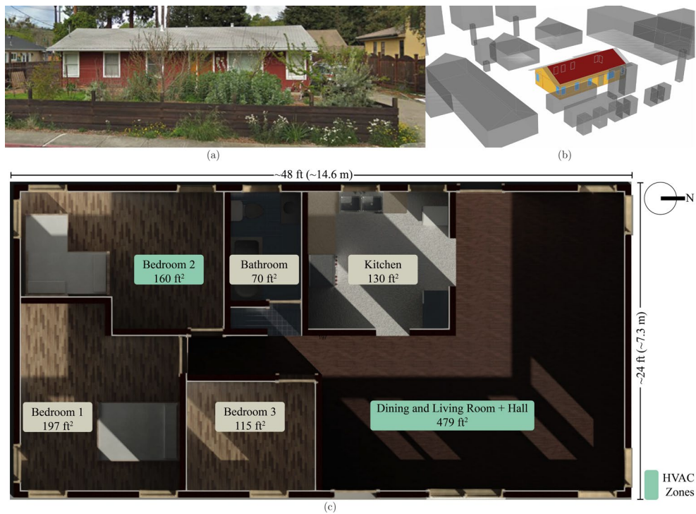
Figure 4: (a) East Façade, (b) 3D Energy Model, and (c) Home Zones (Floor plan distribution).
