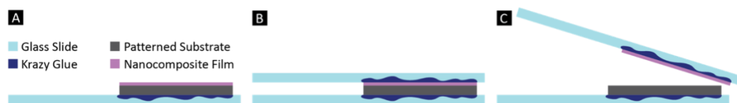
Figure 1-13 Schematic of the film exfoliation process. [A] Krazy Glue KG92548R is used to bond the silicon substrate to glass slide #1, which is later used as a holder. [B] Next, a drop of glue is applied to glass slide #2. The sample is immediately face-down onto the glue droplet. [C] After the glue has completely dried, the glass slides are separated. The nanocomposite sample is exfoliated to glass slide #2. The patterned substrate on slide #1 may be reused.
