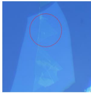
Figure 4-3 image of sample, MoS2 on top of BN
