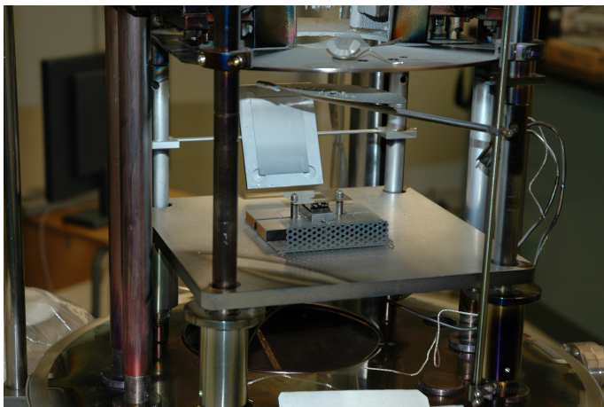
Figure A.26: Crystal loaded onto evaporation jig with shadow mask in place.
