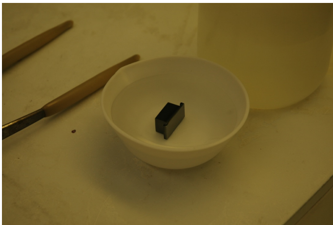
Figure A.5: Detector in HF dip. Note guard ring configuration electrode has been etched away.
