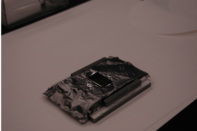
Figure A.19: Weights added to secure Al foil shield.
