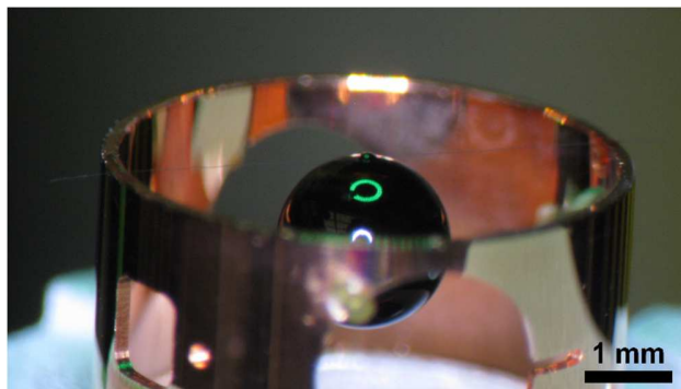
Figure 5. Reinforced CNT yarns support spherical boulders in precision assembled components. A single 6 \mu\text{m} diameter CNT yarn spanning across a circular cylindrical opening is strong enough to easily support a 2 mm diameter sphere that is 600 times its mass glued at the yarn's midpoint with minimal deflection.
