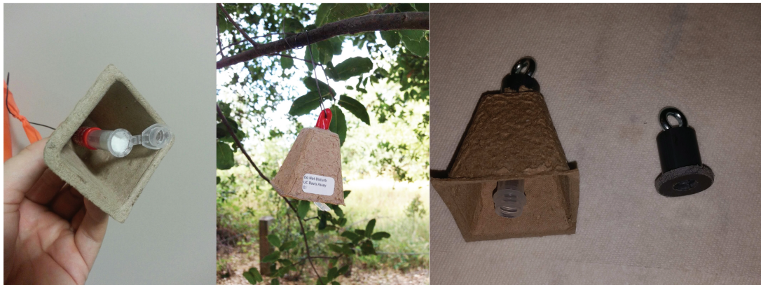
Fig. 1. Photographs of sugar baits. Sugar bait devices were constructed by threading baling wire through a caulking cap and feeding it through the hole of a seedling starter pot. A 2-ml plastic tube (Eppendorf) was filled with ~2 ml of a 40% sucrose and tap water solution and plugged with a cotton dental wick, and this bait tube was inserted into the open end of the caulking cap. Once deployed, the sugar soaked cotton wick was exposed for sugar seeking mosquitoes to access for 6 to 7 d. The image on the right compares the peat pot cover used in SAYO Counties to the small PVC cover used in the COAV.
