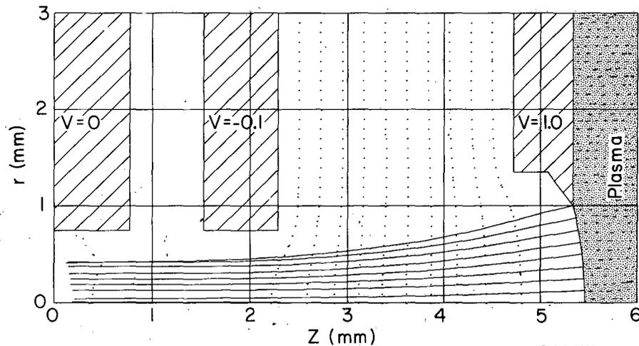
Fig. 1. Electrode geometry for a single-hole circular extractor, showing relative electrode potentials, equipotential contours, and ion trajectories.
