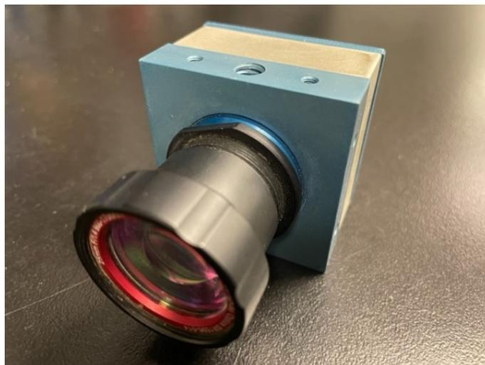
Figure 3.4: The SWIR 640 P-Series, which is a shortwave infrared camera, has also been commonly used for agricultural research. The spectral band is from  $0.9 \mu\text{m}$  to  $1.7 \mu\text{m}$ . The accuracy for the SWIR camera is  $\pm 1 \text{ }^\circ\text{C}$ . It has a resolution of  $640 \times 512$  pixels.
