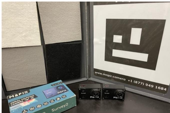
Figure 3.2: The Survey 2 sensors and the reflectance calibration ground target package.
