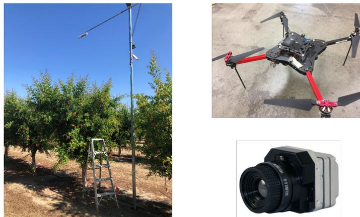
Figure 8.2: The IRT sensor was installed 4.5 m above the soil surface, with a FOV of  $20^\circ$ . A quadcopter was used as the low-cost UAV platform (less than \$1000) to collect high-resolution thermal images at the height of 60 m.
