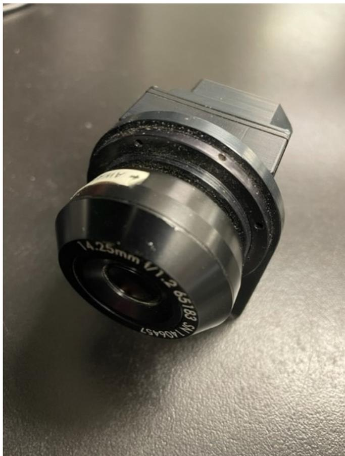
Figure 3.5: The thermal camera has a resolution of  $640 \times 480$  pixels. The spectral band is from  $7 \mu m$  to  $14 \mu m$ . The dimension of the thermal camera is  $34 \text{ mm} \times 30 \text{ mm} \times 34 \text{ mm}$ . The accuracy is designed to be  $\pm 2 \text{ }^\circ\text{C}$ .
