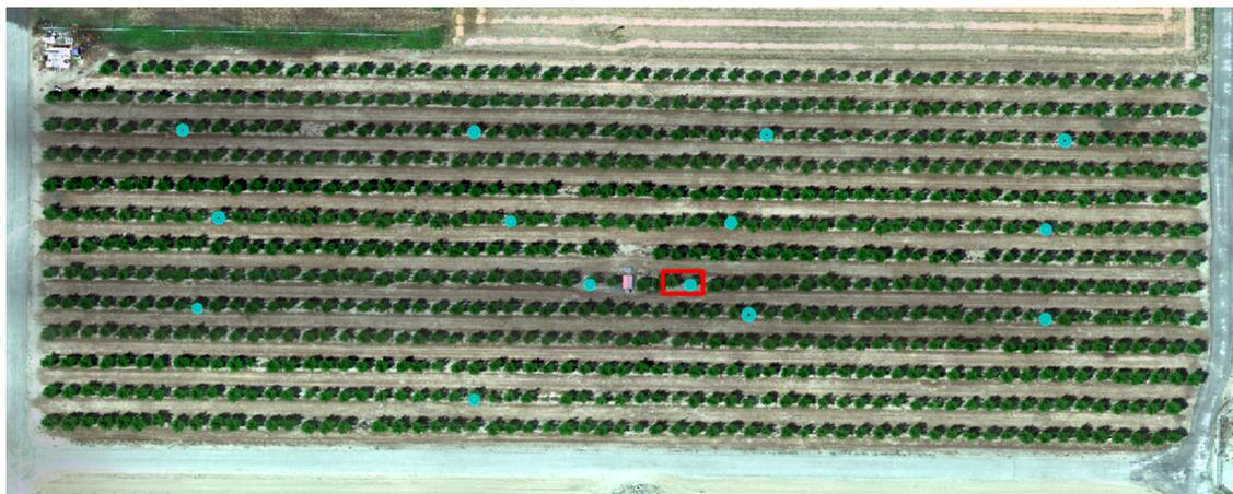
Figure 8.1: The pomegranate field at the USDA-ARS (36.594°N, 119.512°W). The weighing lysimeter is located in the center of the pomegranate field, marked as a red box. The blue marks are where the 14 IRT sensors were installed.
