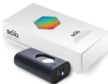
Figure 4.2: A light and small near-infrared spectrometer, Scio. The low power consumption and zero warm up time make it highly responsive and extremely efficient, which allows it to perform hundreds of samplings from a small rechargeable battery. The Scio spectrometer works in NIR at wavelengths of 700 - 1100  $nm$ . It can also be integrated into smart phone as an Edge-AI device.
