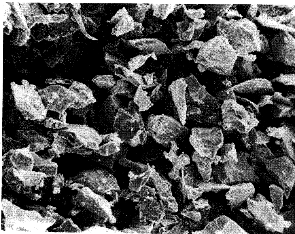
Fig. 10. Scanning electron micrograph of niobium powder.
