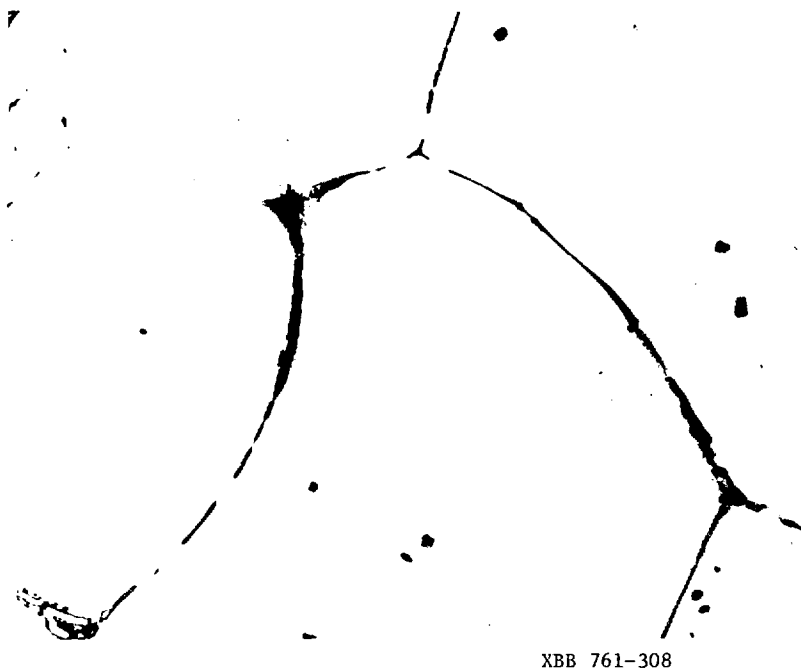
Fig. 6. Anodized arc-melted button of A-15 Nb 3 (Al,Ge); 400x.
