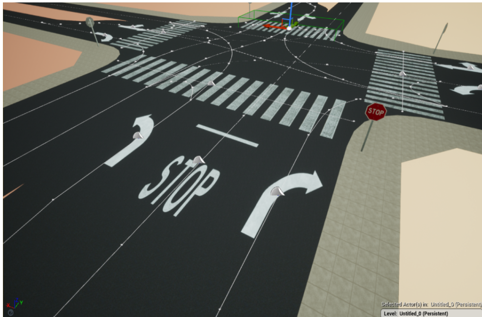
Figure 3.8: Decals can be added to the roads as per the connected lanes at the intersection. In this figure, the nearest decals can be interchanged with other relevant decals as shown in Figure 3.7 and in Figure 3.9.
