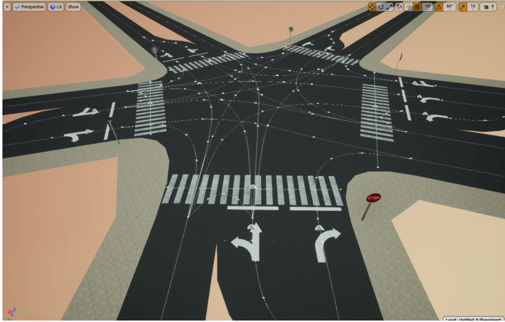
Figure 1.2: A five way intersection generated using Cruzway RoadGen.
