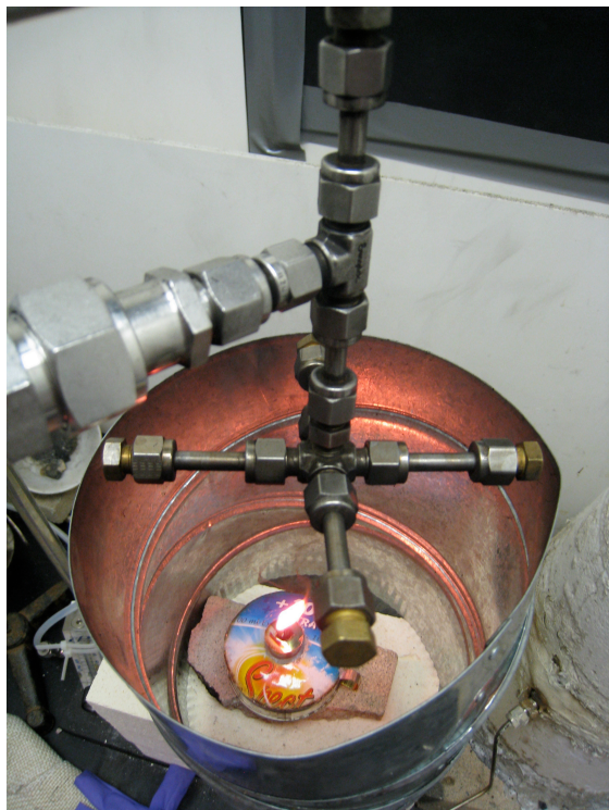
Figure 2.2.2a-b. Laboratory emissions system at the University of Illinois at Urbana-Champaign. Sampling rack (left) and sample probe with lamp (right).
