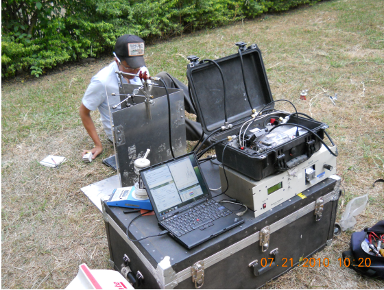
Figures 2.2.4a-b. In-field testing of kerosene lamps in Western Uganda (2010). Sample probe (left) and emissions train (right).
