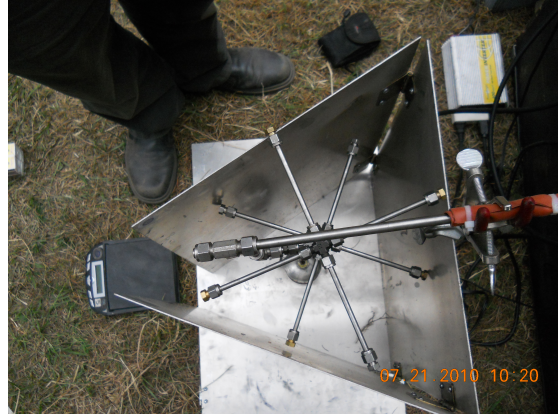
Figures 2.2.4a-b. In-field testing of kerosene lamps in Western Uganda (2010). Sample probe (left) and emissions train (right).
