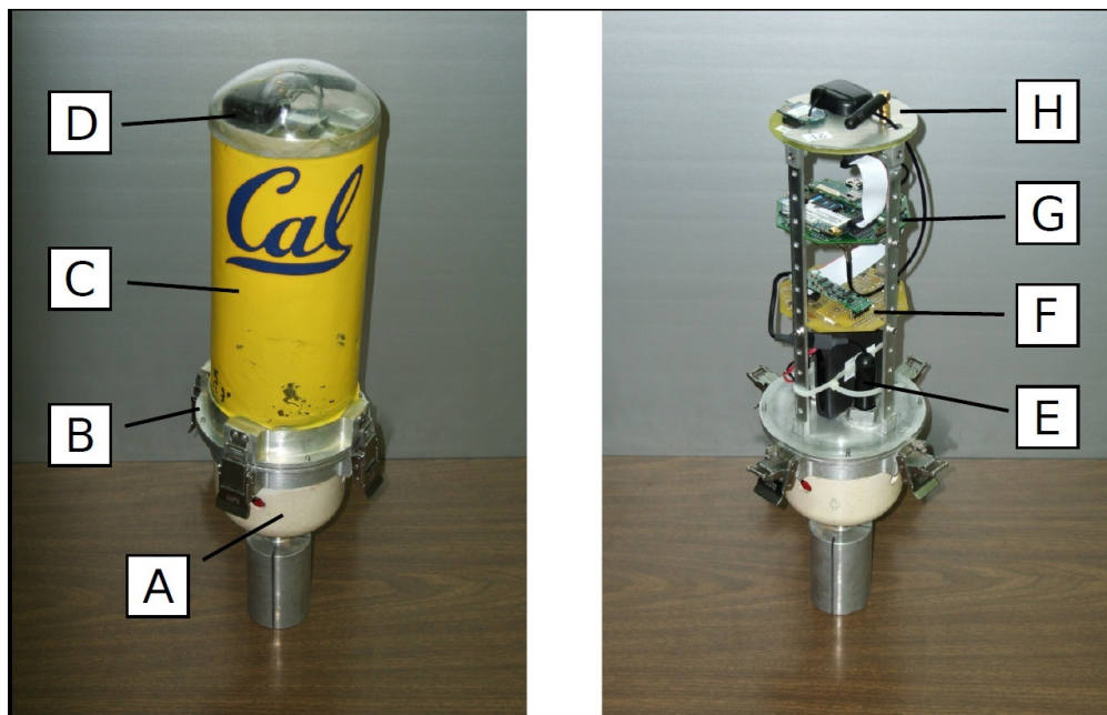
Figure 4.1: Overview of the drifter hull manufactured by the floating sensor network project. Left: closed. Right: open.
