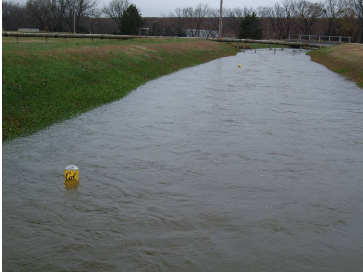
Figure 4.5: Two drifters in the HERU facility supply canal.
