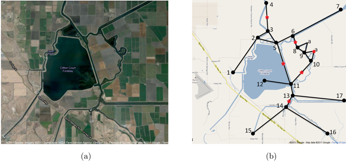
Figure 5.4: (a) Satellite image of the channel network around the Clifton Court Forebay used for the experiment. (b) The network connectivity of the channel network used for the experiment consisting of 19 subchannels, 10 junctions and one reservoir. As boundary conditions, discharge is imposed at nodes 1, 7, 15, 16 and 17 and stage is imposed at nodes 4 and 12 where node 12 represents the reservoir. The red stars show the locations from which flow measurement are obtained for data assimilation.
