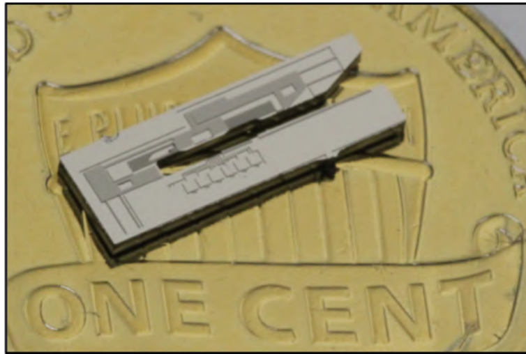
Figure 2.1: A first iteration of the ZIF socket can be seen on top of a gold coated US penny.
