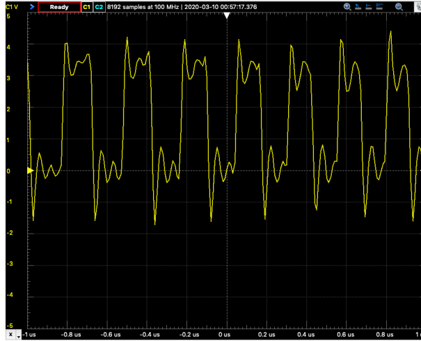
Figure 3.16: The 3.6MHz clock signal seen out of SC \mu M’s GPIO 12 pin.
