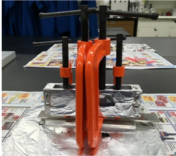
Figure 2-11: C-clamps to apply pressure
