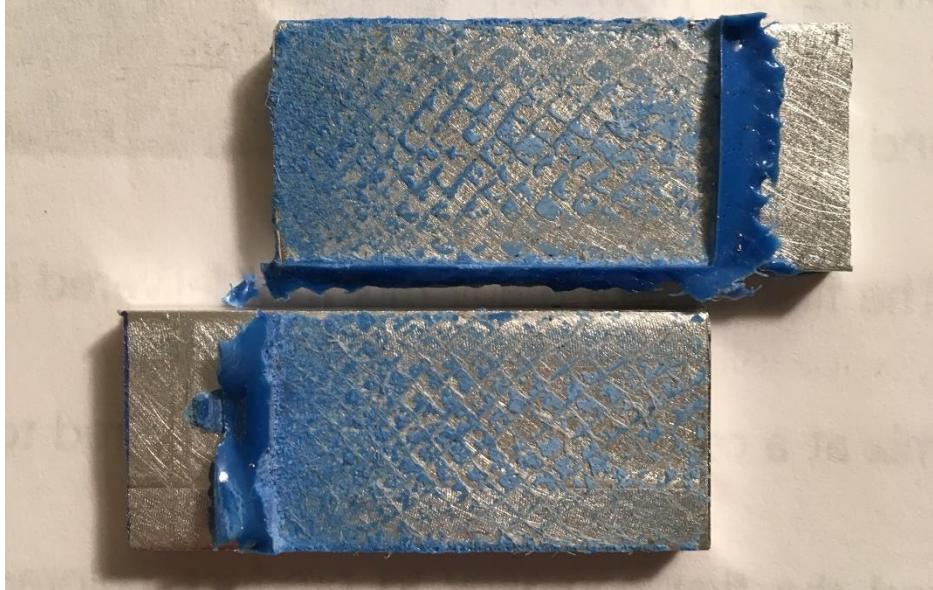
Figure 3-8: SLJ-Sample 3- Fracture Surface
