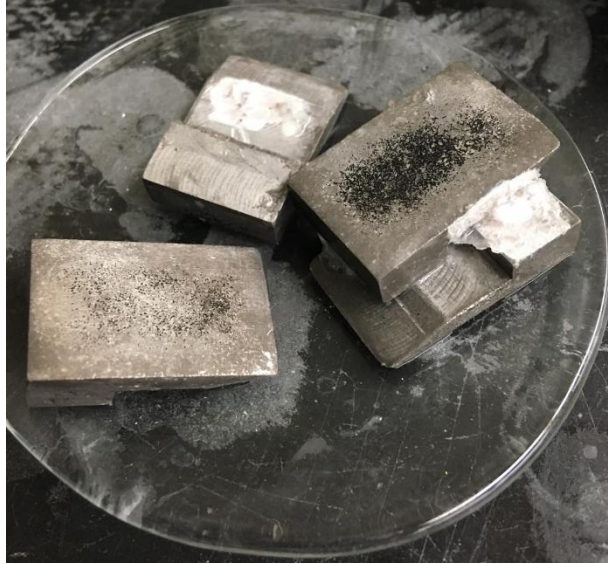
Figure 3-1: Residue from adhesive on the Grip after thermal degradation
