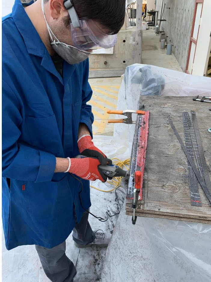
Figure 6-3: Cutting of the cured CFRP laminate
