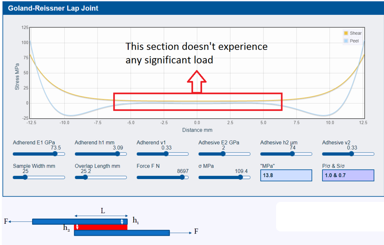
Figure 4-35: Shear & Peel Stress Distributions in a SLJ based on the Goland and Reissner model for a joint with 25.2 mm bondline. The modulus of each substrate is 73.5 GPa. The thickness of each substrate is 3.09 mm. the modulus of the adhesive is 2 GPa. The bondline thickness is 74 μm. the width of the joint is 25 mm. the applied load in this case is 8697 N(Figure modified from the online program [13]).
