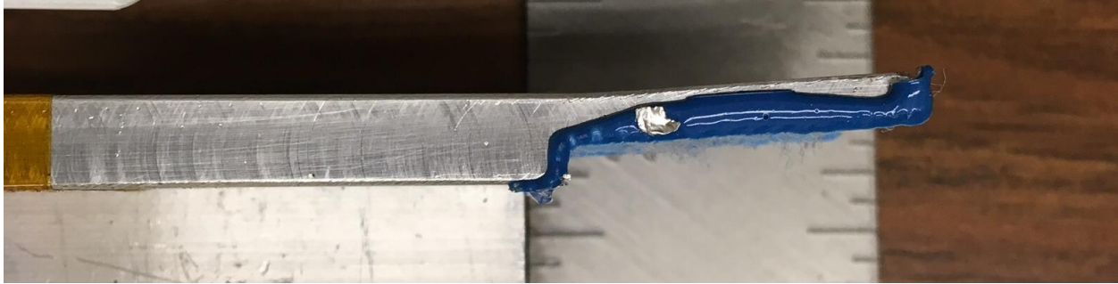
Figure 4-57: Bending contour of substrate #7
