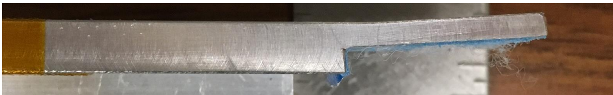
Figure 4-63: Bending contour of substrate #12
