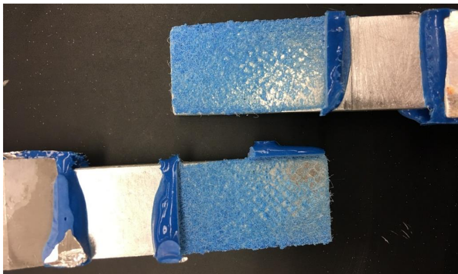
Figure 3-39: SLJ-Sample 11-Fracture Surface
