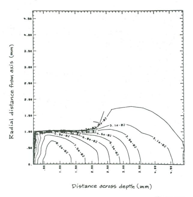
Figure 9. Contour plots of internal temperature in A. Deposition material at  $31\ \mathrm{ns}$  for Case B.
