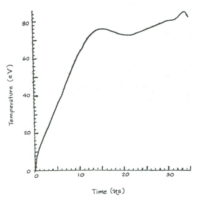
Figure 7. Surface temperature vs. time computed with LASNEX for the spot heating experiment, Case B.
