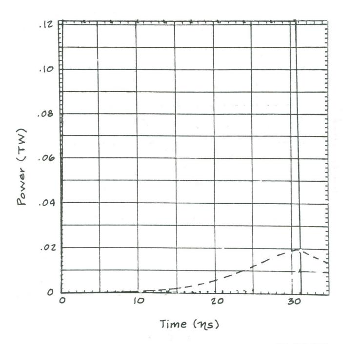
Figure 5. Plot of rate of energy loss from front of disk (dashed curve) versus rate of energy deposition (solid curve) for Case B.
