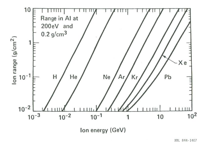
Figure 2. Range-energy plot for ions in hot dense matter
