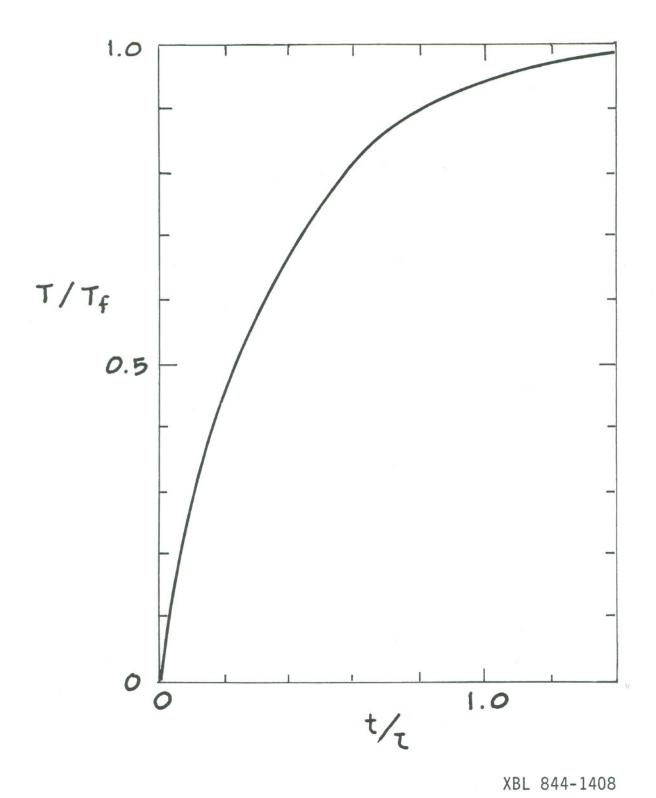
Figure 3. Heating of a disk target by an ion beam. T<sub>f</sub> is the asymptotic limit, where radiation loss equals energy deposited per second. The characteristic time  $\tau$  is defined in text.
