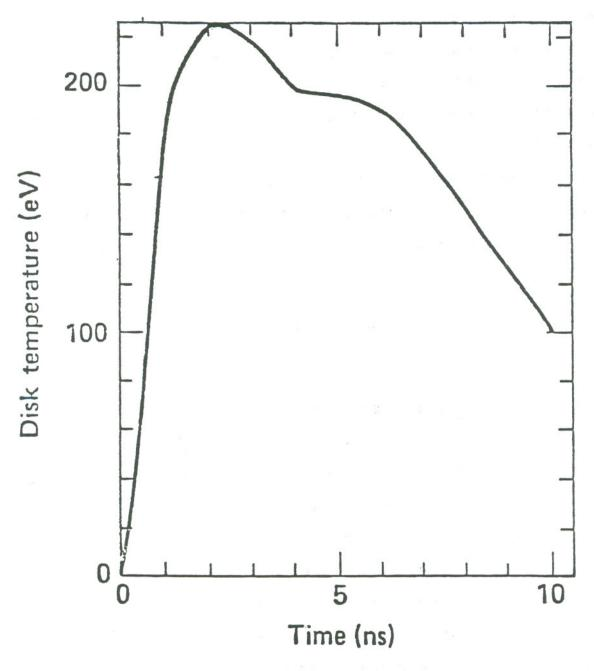
Figure 4. Surface temperature vs. time computed with LASNEX for the spot heating experiment, Case A.
