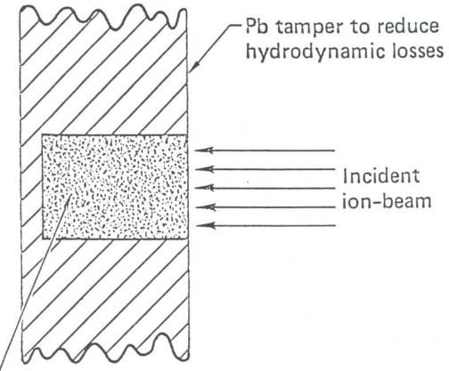
Depositing ions in low density ( $\rho \sim 0.15 \text{ gm/cm}^3$ ) material reduces conversion to longitudinal hydrodynamic motion and ensures that the internal temperature can be readily observed
