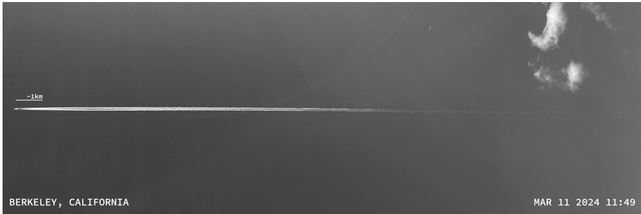
Figure 1.1: Early-stage wake vortices behind cruising aircraft (see left) represented by a pair of long straight-line vortices. The structures are visible far downstream due to surrounding ice crystals from nearby water vapor condensation, also known as contrails. The scale bar in this photo is solely to offer a general sense of the wake vortices’ length scale and is not based on precise quantification.
