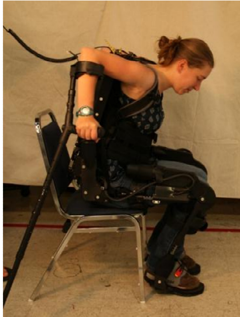
Figure 13-8. The seated position of the sitting maneuver may cause strain on the pilot's shoulders.
