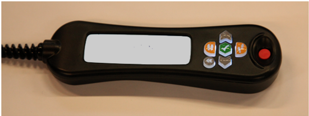
Figure 5-1. The control pad allows the physical therapist to select the state.
