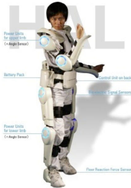
Figure 2-8. HAL is an upper- and lower-body exoskeleton which aids the user's strength. It uses bio-feedback for control.
