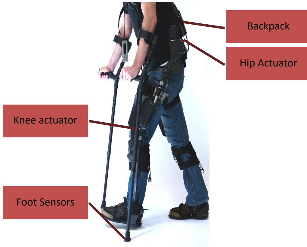
Figure 4-2. The eLEGS robot has four actuators, one at each hip and one at each knee. The foot sensors are located below the sole of the shoe. The backpack supports the computer and batteries.
