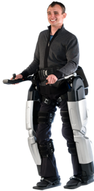
Figure 2-6. Rex, a mobile exoskeleton by Rex-Bionics. Photo from www.rexbionics.com
