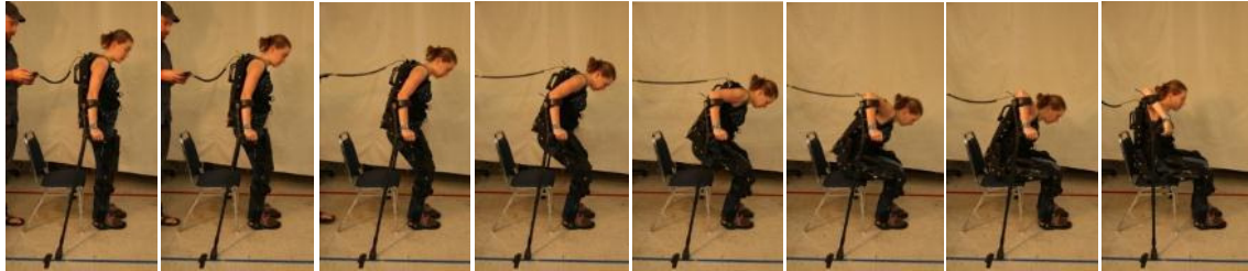
Figure 13-11. The sitting maneuver starts from standing and attempts to keep the center of mass over the feet while sitting.
