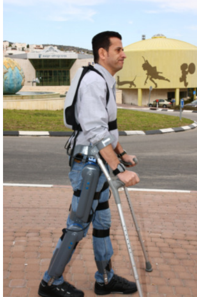
Figure 2-7. ReWalk, a mobile exoskeleton developed by Argo Medical Technologies, is a slim robot which allows a spinal cord injured user to walk. Photo: www.argomedtec.com
