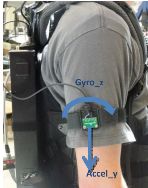
Figure 7-5. The arm sensor case is shown here on a user's arm (without the cover). The sensor is held in place by an elastic band. The accelerometer is oriented down the user's arm. The gyroscope reads the acceleration in the plane of the IMU.
