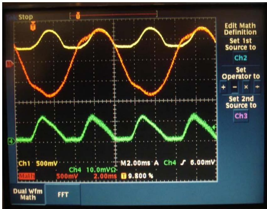
Figure 49 Input Current Waveform for Hybrid Rectifier Circuit with Virtual Junction
