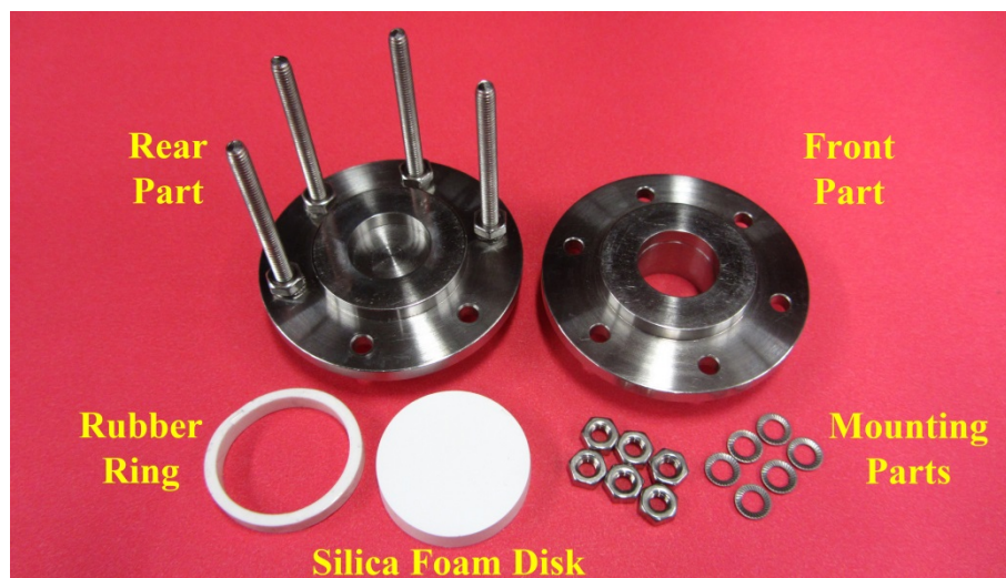
Figure 3.2: The shear promotion support ring and a cellular silica disk sample.
