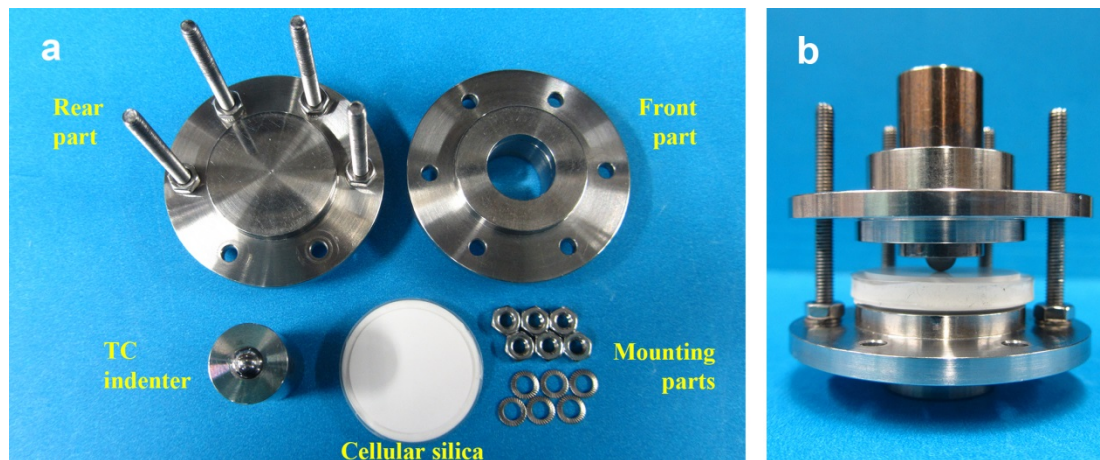
Figure 3.5: Photos of the indentation test system. (a) The system components and a cellular silica sample. (b) A cellular silica sample mounted on the indentation test system.
