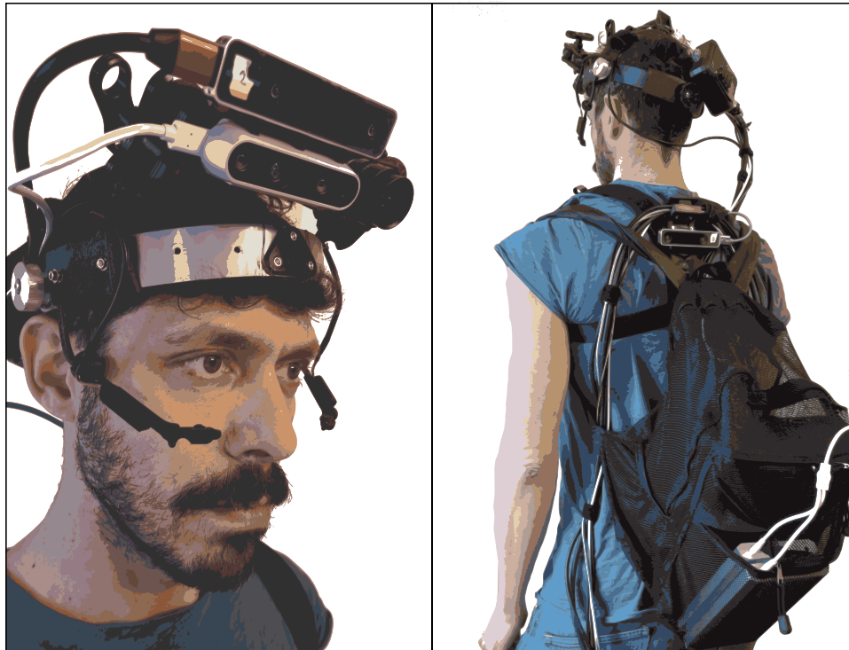
Fig. 3 Subject wearing the device. Left : front view of the subject wearing the headset. The two scene cameras (XIMEA and RealSense D435i) and the tracking camera for the head (RealSense T265) are mounted together with a custom 3D-printed mount, adjustable in position with a three-point ball-and-clamp adjustable mount. Custom ball-and-socket joints combined with set screws enable positioning of eye trackers below the eyes. A white ribbon cable (not visible) connects the XIMEA camera to the rear switch box. Right : rear view of a
