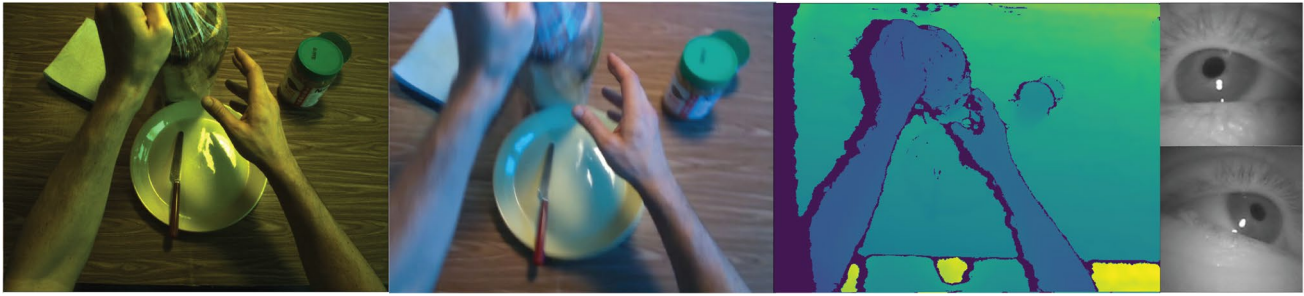
Fig. 1 Left to right : Sample frames collected from XIMEA camera, RealSense D435i RGB stream, RealSense D435i depth stream, and Pupil Labs binocular eye-tracking cameras. Images shown are frames as captured by each sensor, before post-processing
