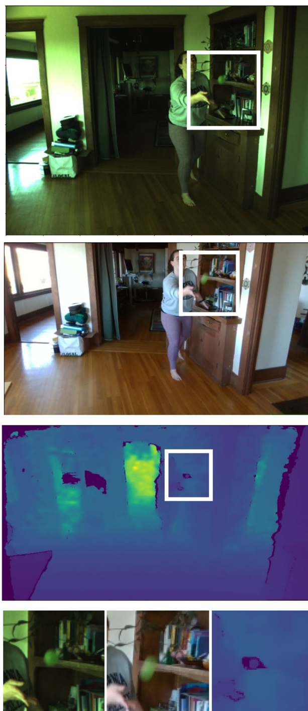
Fig. 7 Visual streams are temporally synchronized to the framerate of the slowest visual stream (60 Hz). Temporally synchronized frames from three visual streams (top to bottom): XIMEA RGB stream, RealSense RGB stream, RealSense depth stream. White boxes indicate zoom-in on bottom panel, showing the ball in same position at moment of release from hand during toss, which is evidence that timestamps are well matched. Note the greater motion blur of the ball in the RealSense RGB stream running at 60 Hz (bottom middle panel) compared to the XIMEA RGB stream running at 200 Hz (bottom left panel)
