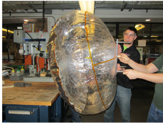
Figure 1.8: S-band inflatable reflector antenna developed for 3U CubeSat [46]. The stowed volume of this antenna 0.2U.
