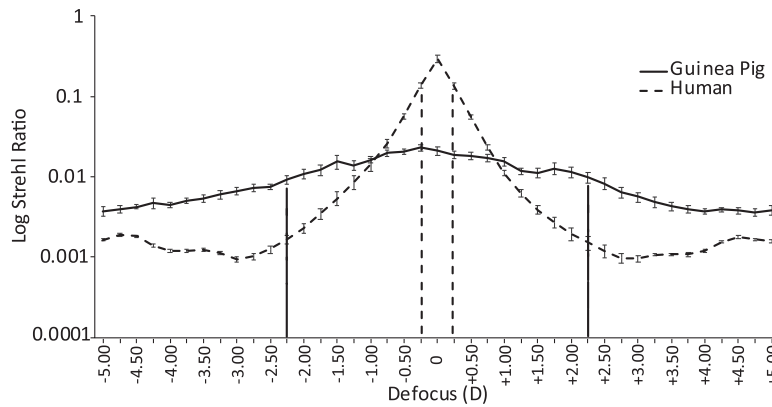
FIGURE 4. Through-focus estimation of depth of focus (DOF) derived from Strehl ratios centered around their respective peaks. The DOF estimated for seven guinea pig eyes was 4.50 D (–2.25 to +2.25 D), much larger than the estimated DOF for 18 human eyes, 0.50 D (–0.25 to +0.25 D). Error bars represent the standard errors of the mean. Calculations used a 4-mm pupil and 550-nm wavelength.
