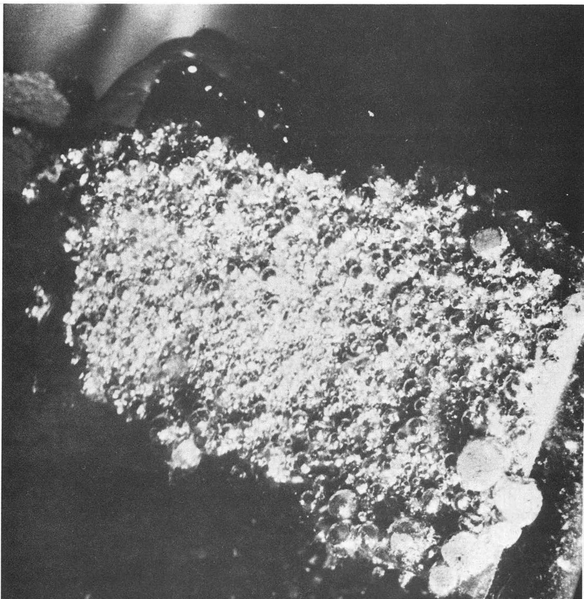
Figure 7-3. Potassium deposit from 1.0 m \text{KAlCl}_4/\text{PC} on a platinum electrode with soft glass coated edges, 70-85°C, 0.3 \text{mA}/\text{cm}^2 , 10X.
