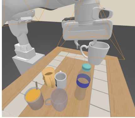
Figure 2.7: Unstable antipodal grasp. All points between the parallel gripper were considered in the grasp cost function.
