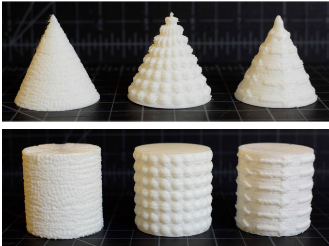
Figure 6. 3 cylinders and 3 cones printed with alligator (indexical), bump (iconic), and arrow (symbolic) textures, respectively.
