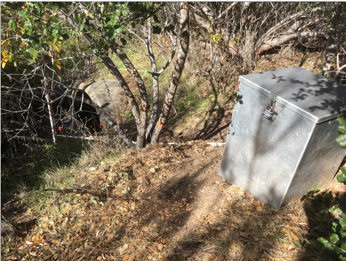
A stormwater sample collection system recently installed on a tributary that drains into NCOS and Devereux Slough.
