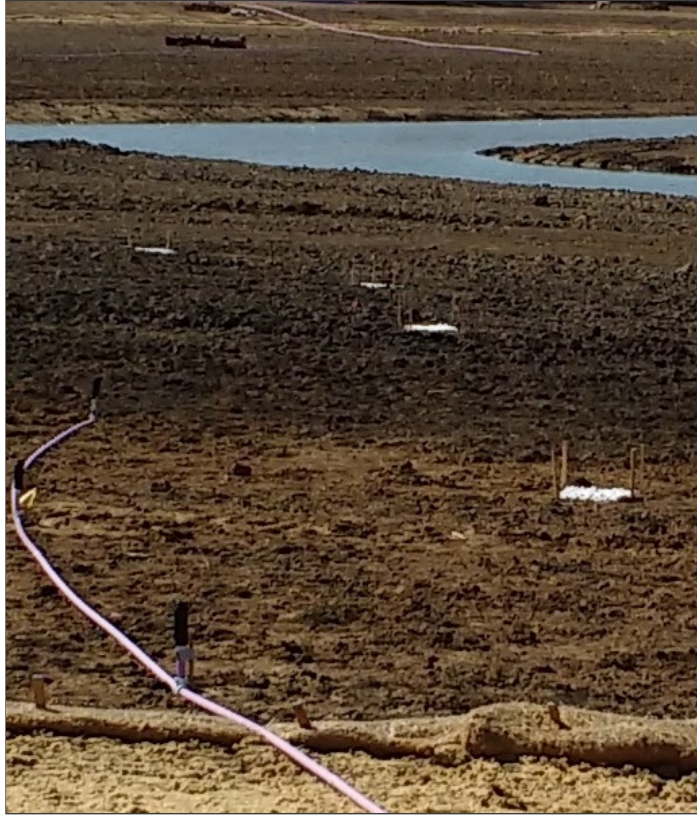
Examples of feldspar plots for monitoring sediment accretion in Devereux Slough.
