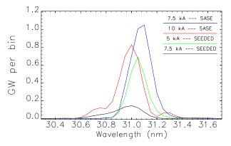
Figure 5: Predicted (GINGER calculations) output spectra at the 31-nm wavelength fundamental for the various SASE and seeded cases. Each bin is  $64.6 \, \text{meV}$  wide while 1 GW is equivalent to  $1.0 \times 10^{13} \, \text{photons}$ .
