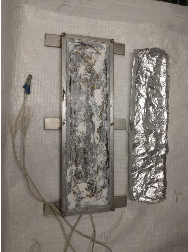
Figure A.1.1: Sample plate construction as seen from the top with an aluminum sample vessel next to it (left) and with the sample plate opened (right) to reveal the heating element, location of embedded temperature sensor, and Teflon seal.
