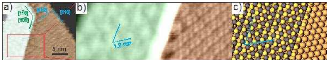
Fig 2.2 (a) portion of a MoS 2 layer (left, green) on a sulfur terminated Cu(111) terrace with a dislocation step indicating substrate crystallographic axes. (b) Enlarged portion near the MoS 2 edge showing angular registry between MoS 2 Moiré pattern and straight edge. (c) atomic model of b highlighting the 1.3 nm Moiré pattern visible in (b). MoS 2 drawn as sulfur terminated; no substrate sulfur superstructure included. Image Parameters: Bias: -560 mV, Current: 140 pA.
