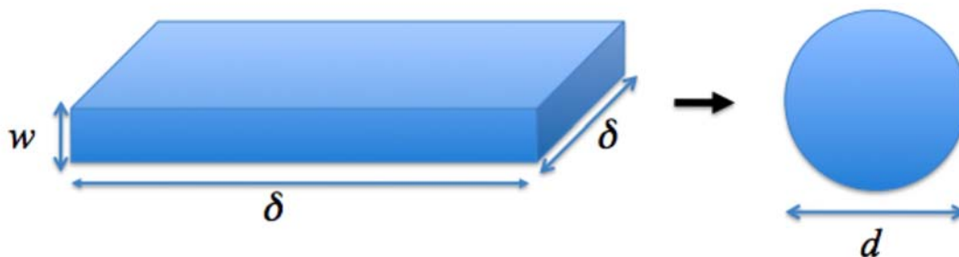
Fig. 14. Geometry of assumed square patch of foil that transforms into a spherical droplet due to differential surface tension.
