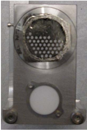
Fig. 8. Target holder containing a platinum target foil (above) and a small scintillator (below).
