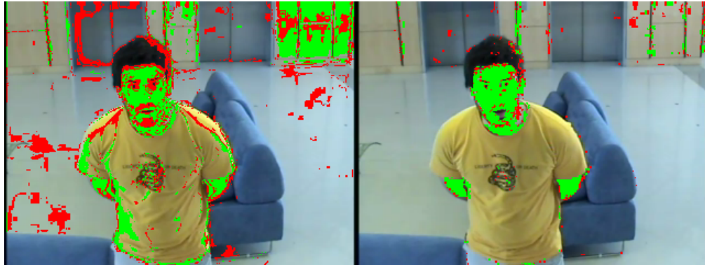
Figure 2.8: Results of the skin-color detector after several iterations of training. Left image is the result after 1 iteration and right image is the results after several iterations of active training. Green pixels indicate skin regions with high confidence and red pixels indicate predicted skin regions, yet with lower confidence.
