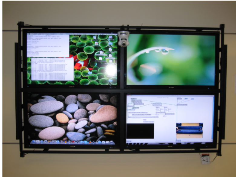
Figure 2.1: A frontal view of TAC display unit. The position of the PTZ camera and four of the microphones are shown.
