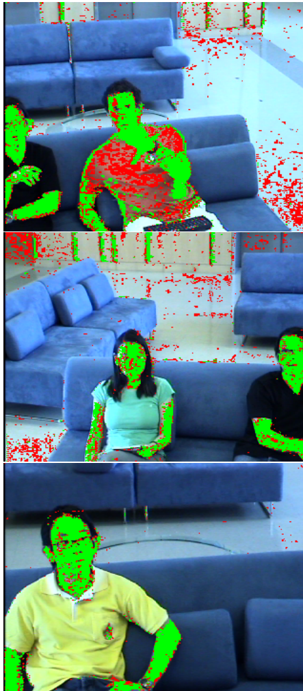
Figure 2.7: Results of the skin-color detector after the first iteration of active training. Green pixels indicate skin regions with high confidence and red pixels indicate predicted skin regions, yet with lower confidence.
