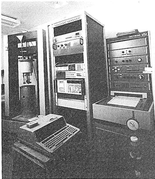
Fig. 4 Mechanical facility for compression and thermal tests (400 to 4 K).
