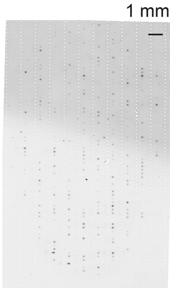
Figure 2.3: Characterization of electromigration uniformity. Inverted micrograph of TurboGFP-expressing U373 cells assayed with the (sc)^2WB for TurboGFP after cytoplasm-specific lysis. TurboGFP-expressing U373 cells were settled into the (sc)^2WB device. The cytoplasmic lysis buffer was applied for 25 s. An electric field ( 40 \text{ V cm}^{-1} ) was applied for 17 s immediately following the completion of lysis. The TurboGFP average peak center location x = 397.0 \pm 25.4 \mu\text{m} ( n = 187 ), which yields a coefficient of variation, CV = 6.4\% .
