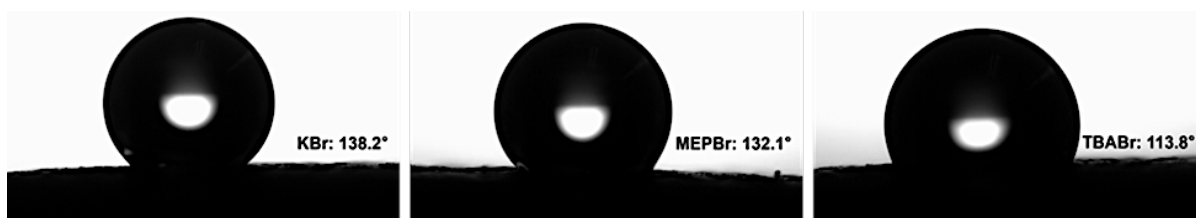
Figure 38. Contact angle of test electrolyte on the surface of a porous activated carbon pellet. (left) aqueous KBr solution droplet; (middle) aqueous MEPBr solution droplet; (right) aqueous TBABr solution droplet.
