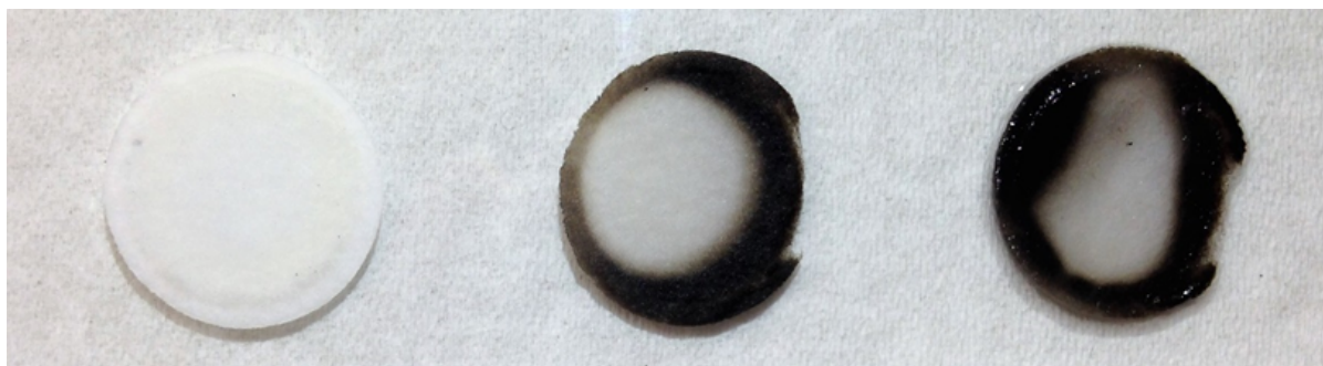
Figure 43. Paper separators after GCD cycling. (left) separator from asymmetric KBr/TBABr cell; (middle) separator from asymmetric KBr/MEPBr cell; (right) separator from asymmetric KBr cell.
