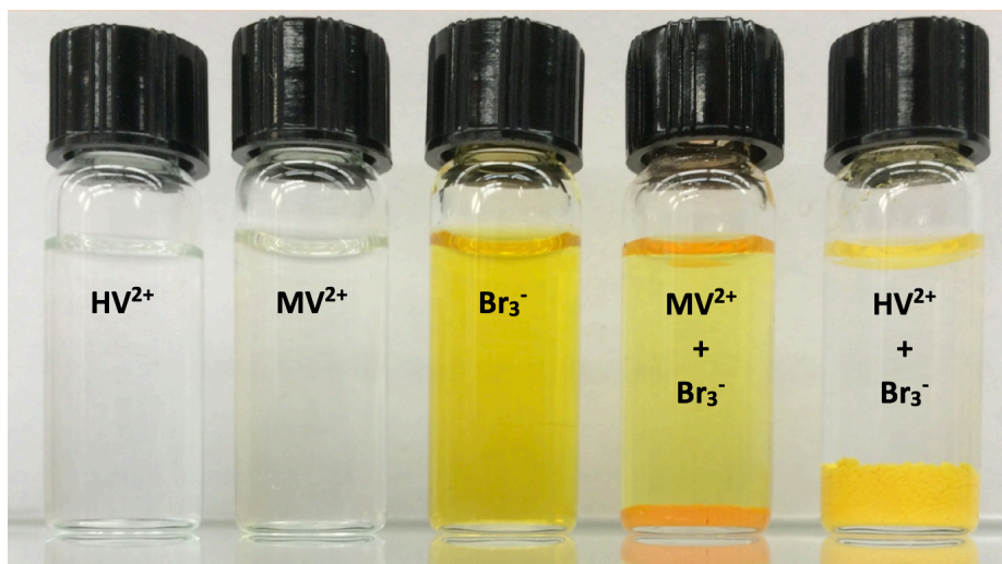
Figure 30. Complexation of \text{Br}_3^- by methyl and heptyl viologen dications. 20 mM \text{MVCl}_2 or \text{HVBr}_2 (left) and 40 mM \text{Br}_3^- (center) form solid complexes of [\text{MV}^{2+}\cdot 2\text{Br}_3^-] or [\text{HV}^{2+}\cdot 2\text{Br}_3^-] (right) when mixed in aqueous solution. The degree of complex precipitation is higher for HV than for MV. In the case of MV, a
