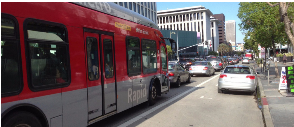
Parked vehicles disrupt TTL operation, as such planning for pre- and post-implementation strategies is important. Image courtesy of Streetsblog LA (5/15/2015).
