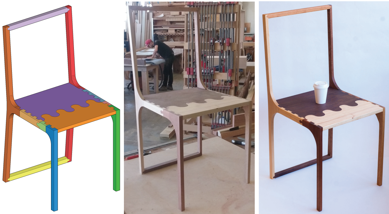
Figure 3.14: We commissioned a woodworker to fabricate a version of the Branca chair at full size using the solid 3D parts generated by our tool. (Coffee cup was added for scale.)
